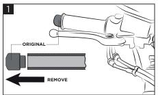
Untighten the original screw and remove the counterweight.
