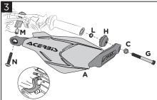
Fix the handguard (A) to the handlebar using the the washer (L), the spacer (H), the bushing (C) and the screw (G) as shown in the figure. Fix the bar to the bracket using the screw (N) and the bushing (M).
